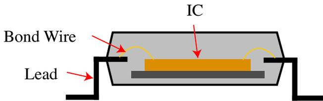
Figure 1: Classic IC lead-frame package.
