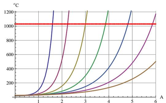
Figure 3: Au-wire current capacities for diameters  $D_w = \{0.8, 1.0, \dots, 1.8, 2.0\}$  mil and  $L_w = 2.5$  mm. The plotted temperature is at the wire mid-point, where the hottest point is expected.
